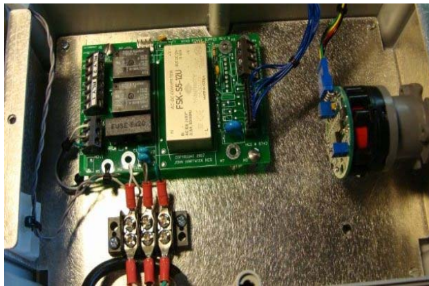
O2 POWER SUPPLY BOARD (A.1)
